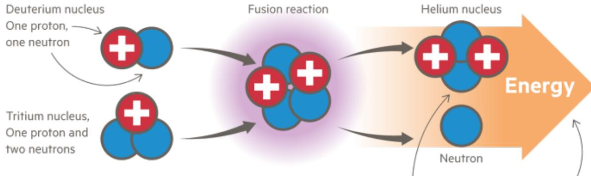
Typically the hydrogen isotopes deuterium and tritium are used because they fuse at relatively lower temperatures and release a lot of energy. Deuterium is found in seawater, while tritium can be extracted from lithium
